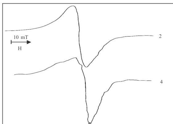
Fig. 1 X-band EPR spectra of complexes (2) and (4) on polycrystalline samples at room temperature
